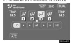
The outlets from which air is delivered can be selected manually by touching the touch-screen button. The function of each mode is as follows:
