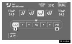
▶ 1 Fan speed at low2 Fan speed at high
