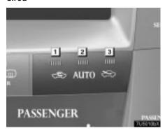
Each time you push the air intake control button, the mode changes in order from the RECIRCULATED AIR mode to AUTO-MATIC mode to OUTSIDE AIR mode, then back to the RECIRCULATED AIR mode. Each indicator light shows which mode is now selected.
