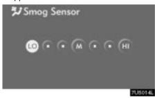
The sensitivity of the touch-screen button is set to be higher toward "HI" and lower toward "I O".
