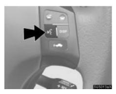
By pushing the switch above, you can operate the speech command system.
