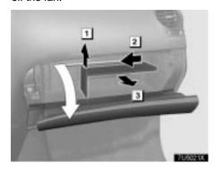
3. Open the glove box. Lift and remove the partition.
