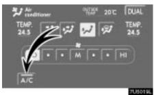
Touch "A/C" to turn the air conditioning on and touch it again to turn the air conditioning off. If you turn off the air conditioning manually, the EXHAUST GAS AUTOMATIC mode will be cancelled.
