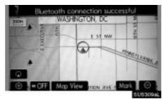
When the engine switch is in "ACC" or "IG-ON" mode, the selected Bluetooth® phone will be automatically connected and the connection result is displayed.
