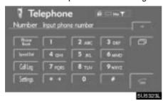
Touch the desired key to input the telephone number.
