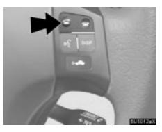
By pushing the telephone switch above, you can receive a call or hang up without taking your hands off the steering wheel.
