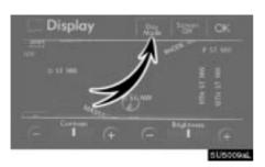
Depending on the position of the headlight switch, the screen changes to the day mode or night mode.
