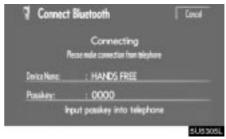
6. When this screen is displayed, input the Passkey displayed on the screen into the phone.
