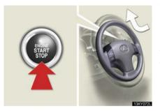
When the engine switch is turned OFF, the steering wheel returns to its stowed position by moving up and away to enable easier driver entry and exit.
