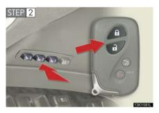
Press and hold the desired button (1, 2 or 3) while pressing the or button on the wireless remote control until the signal beeps.
