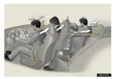
The pretensioner helps the seat belt to quickly restrain the occupant by retracting the seat belt when the vehicle is subjected to certain types of severe frontal collision.
