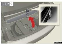
Secure the panel using the hook provided.
