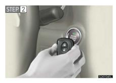
Hold the electronic key close to the engine switch (within 0.4 in. [10 mm]). Make sure that the button side of the key is facing away from the engine switch.
