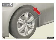
Slightly loosen the wheel nuts (one turn).
