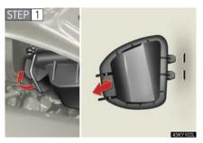
Release the lock and remove the cover.
