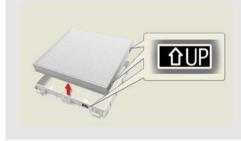
Remove the air conditioning filter from the filter case and replace it with a new one.
