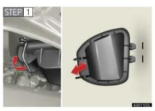
Release the lock and remove the cover.
