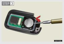
Remove the depleted battery.
