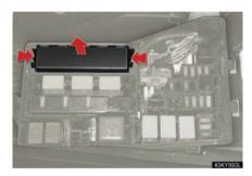
Lift the lid off while pushing the tabs on either side.
