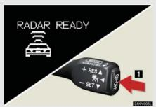
Selecting vehicle-to-vehicle distance control mode
