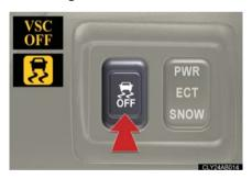
Push and hold the button for more than 3 seconds while the vehicle is stopped to turn off TRAC/VSC.
