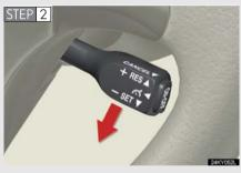
Accelerate or decelerate to the desired speed and press the lever down to set the cruise control speed.
