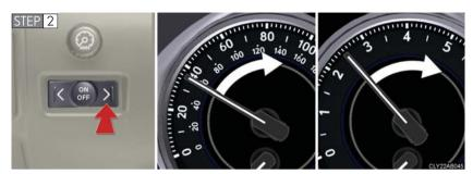
Push the < or > switch within 6 seconds of the speedometer or tachometer needle moving to change the setting of the desired speed, then turn the indicator mode to ON by pushing the ON/OFF button.
