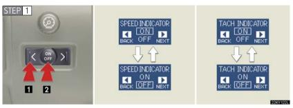
Push the < or > switch to select the speed or tacho indicator set mode. (1) Turn the speed or tacho indicator to OFF and then ON by pushing the ON/OFF button. (2)
