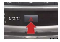
Engaging the emergency flasher switch causes all the turn signal lights to flash.
