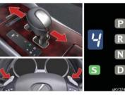
2 To upshift: shift the shift lever toward "+", or pull the "+" shift paddle switch on the steering wheel toward the driver.
