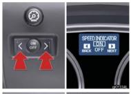
1 To cycle through the functions, press either the left or right selector switch.
