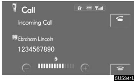
When a call is received, this screen is displayed with a sound. Touch or push of the steering wheel to talk on the phone.
