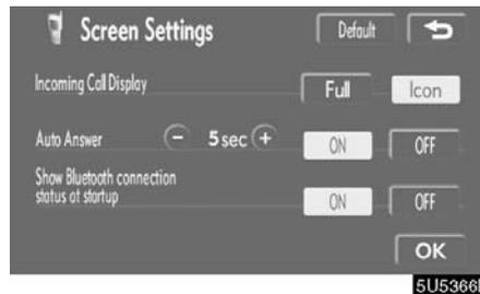
When the engine switch is in “ACC” or “IG-ON” mode and the Bluetooth is automatically connected, the connection check is displayed.
