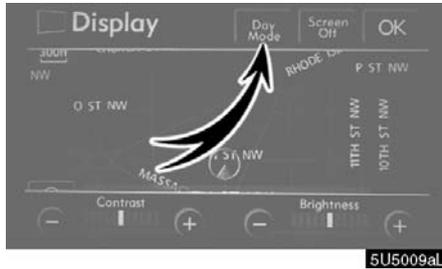
Depending on the position of the headlight switch, the screen changes to the day mode or night mode.
