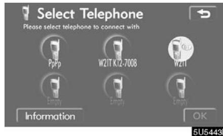
Although you can register up to 6 Bluetooth phones in the system, only one Bluetooth phone can function at a time.
