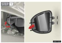
Release the lock and remove the cover.
