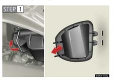
Release the lock and remove the cover.
