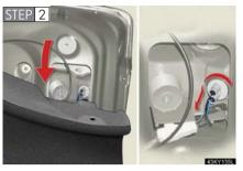
Partly remove the trunk panel cover and turn bulb bases counterclockwise.
