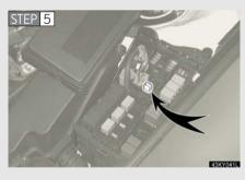
Remove the fuse with the pullout tool.
