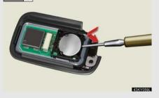
Remove the depleted battery.
