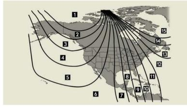
The direction display deviates from the true direction determined by the earth's magnetic field. The amount of deviation varies according to the geographic position of the vehicle.
