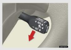
Accelerate or decelerate to the desired speed and press the lever down to set.
