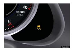
If the vehicle is in danger of slipping, rolling backwards when starting on an incline, or if the rear wheels spin, the slip indicator light flashes to indicate that the VSC/ TRAC/hill-start assist control systems have been engaged.
