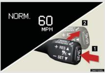
Selecting vehicle-to-vehicle distance control mode
