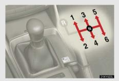
Fully depress the clutch pedal before operating the shift lever.
