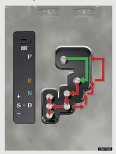
While the engine switch is in IG-ON mode, depress the brake pedal and move the shift lever.
