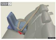
Run the seat belt through the infant seat and insert the plate into the buckle. Make sure that the belt is not twisted.
