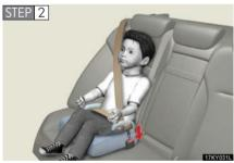
Sit the child in the child seat. Fit the seat belt to the child seat according to the manufacturer's instructions and insert the plate into the buckle. Make sure that the belt is not twisted.
