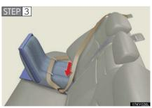
Fully extend the shoulder belt and then allow it to retract slightly in order to activate the ALR lock mode.
