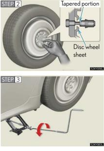
Install the spare tire and loosely tighten each nut by hand to approximately the same amount.
