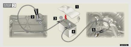
Connecting the jumper cables.
