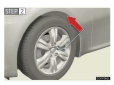
Slightly loosen the wheel nuts (one turn).
