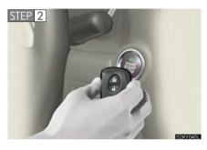
Hold the electronic key close to the engine switch (within 0.4 in. [10 mm]). Make sure that the button side of the key is facing away from the engine switch.
