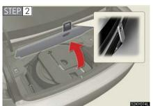
Secure the panel using the hook provided.
