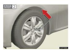
Slightly loosen the wheel nuts (one turn).
