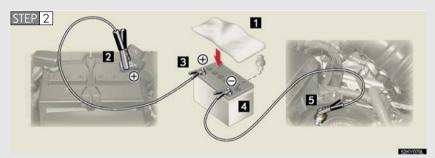
Connecting the jumper cables.
