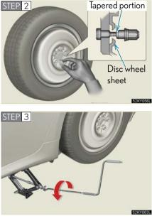
Install the spare tire and loosely tighten each nut by hand to approximately the same amount.
