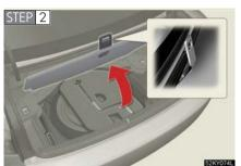
Secure the panel using the hook provided.
