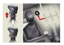
To operate the shift lever, the clutch pedal must be fully depressed.
